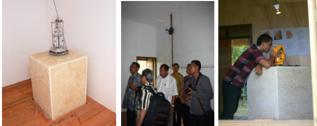
FGE and GSM 90-F1 are placed in the Variation Room, and a measurement which is taken in the Absolute House using DI-flux magnetometer and non-magnetic Theodolite.
