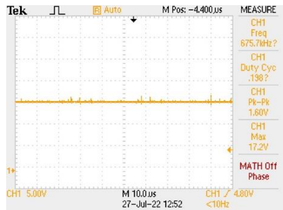
Fig. 7. Sepic Converter Output Voltage.
