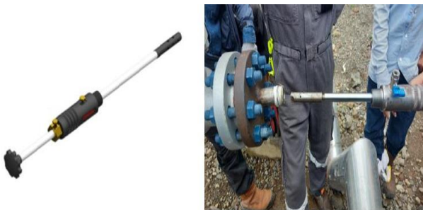
Fig. 11. Scale/corrosion coupon used in Well-A for the DSI project.
